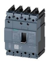
circuit breaker 3VA5 UL frame 125 breaking capacity class S 25kA @ 480V 4-pole, line protection TM210, FTFM, In=100A overload protection Ir=100A fixed short-circuit protection Ii=10 x In N conductor protection 100% without connection
