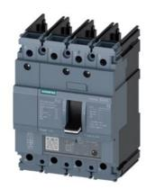
circuit breaker 3VA5 UL frame 125 breaking capacity class S 25kA @ 480V 4-pole, line protection TM230, FTAM, In=100A overload protection Ir=100A fixed short-circuit protection Ii=5...10 x In N conductor protection 100% without connection
