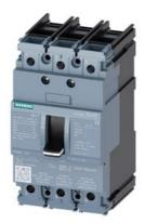
molded case switch 3VA5 UL frame 125 max. sh-circ breaking capacity 65kA @ 480 V 3-pole, line protection MCS110, In=100A without overload protection self-protection li=16 x In cable connection on both sides
