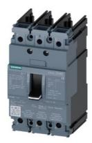
molded case switch 3VA5 UL frame 125 max short-circuit curr. rating 65kA @ 480 V 3-pole MCS110, In=100A without overload protection SELF PROTECTION li=16 x In Al-lug, line side
