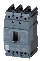
molded case switch 3VA5 UL frame 125 max. sh-circ breaking capacity 65kA @ 480V 3-pole, line protection MCS110, In=100A without overload protection self-protection li=16 x In without connection
