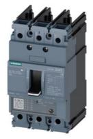
circuit breaker 3VA5 UL frame 125 3-pole, starter protection TM120M, AM, In=3A without overload protection short-circuit protection Ii=3...7 x In without connection
