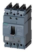
circuit breaker 3VA5 UL frame 125 3-pole, starter protection TM120M, AM, In=2A without overload protection short-circuit protection Ii=3...7 x In without connection
