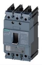
circuit breaker 3VA5 UL frame 125 3-pole, starter protection TM120M, AM, In=2A without overload protection short-circuit protection Ii=5...12 x In without connection
