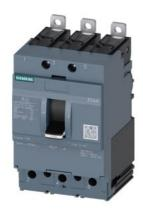
circuit breaker 3VA4 UL frame 125 breaking capacity class M 35kA @ 480 V 3-pole, line protection TM210, FTFM, In=90A overload protection Ir=90A fixed short-circuit protection Ii=10 x In UL489 SB (naval), 50 deg. cel. clamp connection
