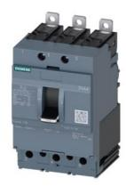
circuit breaker 3VA4 UL frame 125 breaking capacity class M 35kA @ 480 V 3-pole, line protection TM210, FTFM, In=90A overload protection Ir=90A fixed short-circuit protection Ii=10 x In clamp connection
