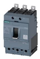
circuit breaker 3VA4 UL frame 125 breaking capacity class H 65kA @ 480 V 3-pole, line protection TM210, FTFM, In=70A overload protection Ir=70A fixed short-circuit protection Ii=10 x In UL489 SB (naval), 50 deg. cel. clamp connection
