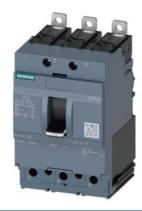
circuit breaker 3VA4 UL frame 125 breaking capacity class H 65kA @ 480 V 3-pole, line protection TM210, FTFM, In=70A overload protection Ir=70A fixed short-circuit protection Ii=10 x In clamp connection
