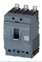
circuit breaker 3VA4 UL frame 125 breaking capacity class M 35kA @ 480 V 3-pole, line protection TM210, FTFM, In=70A overload protection Ir=70A fixed short-circuit protection Ii=10 x In UL489 SB (naval), 50 deg. cel. clamp connection
