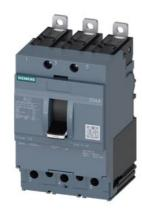
circuit breaker 3VA4 UL frame 125 breaking capacity class H 65kA @ 480 V 3-pole, line protection TM210, FTFM, In=40A overload protection Ir=40A fixed short-circuit protection Ii=10 x In UL489 SB (naval), 50 deg. cel. clamp connection
