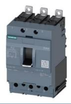
circuit breaker 3VA4 UL frame 125 breaking capacity class H 65kA @ 480 V 3-pole, line protection TM210, FTFM, In=40A overload protection Ir=40A fixed short-circuit protection Ii=10 x In clamp connection
