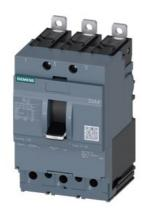
circuit breaker 3VA4 UL frame 125 breaking capacity class M 35kA @ 480 V 3-pole, line protection TM210, FTFM, In=40A overload protection Ir=40A fixed short-circuit protection li=10 x In clamp connection
