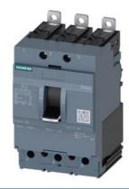
circuit breaker 3VA4 UL frame 125 breaking capacity class H 65kA @ 480 V 3-pole, line protection TM210, FTFM, In=35A overload protection Ir=35A fixed short-circuit protection Ii=10 x In clamp connection
