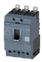
circuit breaker 3VA4 UL frame 125 breaking capacity class H 65kA @ 480 V 3-pole, line protection TM210, FTFM, In=25A overload protection Ir=25A fixed short-circuit protection Ii=12 x In UL489 SB (naval), 50 deg. cel. clamp connection
