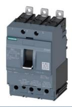
molded case switch 3VA4 UL frame 125 max. sh-circ breaking capacity 65kA @ 480 V 3-pole, line protection MCS110, In=100A without overload protection self-protection li=16 x In clamp connection
