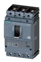
circuit breaker 3VA2 IEC frame 160 breaking capacity class C Icu=110kA @ 415V 3-pole, motor protection ETU350M, LSI, In=63A overload protection Ir=25A...63A short-circuit protection Isd=3...15 x Ir, Ii=15 x In nut keeper kit
