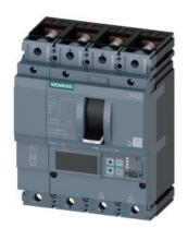
circuit breaker 3VA2 IEC frame 160 breaking capacity class C Icu=110kA @ 415V 4-pole, line protection ETU860, LSIG, In=63A overload protection Ir=25A...63A short-circuit protection Isd=0.6..10x In, Ii=1.5..12x In N conductor protection adjustable (OFF, up to 160%) gr.-fault prot., can be sw. off Ig=0.25...1 x In= tg=0.05-0.8s nut keeper kit
