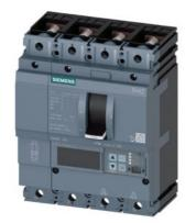
circuit breaker 3VA2 IEC frame 160 breaking capacity class C Icu=110kA @ 415V 4-pole, line protection ETU850, LSI, In=63A overload protection Ir=25A...63A shortcircuit protection Isd=0.6..10x In, Ii=1.5..12x In N conductor protection adjustable (OFF, up to 160%) nut keeper kit
