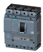
circuit breaker 3VA2 IEC frame 160 breaking capacity class C Icu=110kA @ 415V 4-pole, line protection ETU350, LSI, In=63A overload protection Ir=25A...63A short-circuit protection Isd=1.5...10 x Ir, Ii=12 x In N conductor protection adjustable (OFF, 100%) clamp connection
