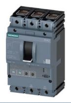
circuit breaker 3VA2 IEC frame 160 breaking capacity class C Icu=110kA @ 415V 3-pole, line protection ETU350, LSI, In=63A overload protection Ir=25A...63A short-circuit protection Isd=1.5...10 x Ir, Ii=12 x In clamp connection
