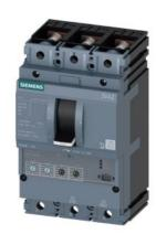
circuit breaker 3VA2 IEC frame 160 breaking capacity class C Icu=110kA @ 415V 3-pole, line protection ETU350, LSI, In=63A overload protection Ir=25A...63A short-circuit protection Isd=1.5...10 x Ir, Ii=12 x In nut keeper kit
