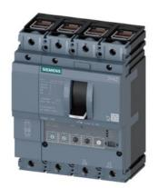
circuit breaker 3VA2 IEC frame 160 breaking capacity class C Icu=110kA @ 415V 4-pole, line protection ETU330, LIG, In=63A overload protection Ir=25A...63A short-circuit protection Ii=1.5...12 x In N conductor protection adjustable (OFF, 100%) ground-fault protection Ig=0.25...1 x In= tg=0.1/0.3s clamp connection
