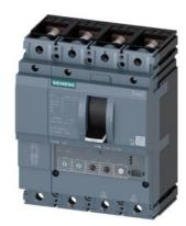
circuit breaker 3VA2 IEC frame 160 breaking capacity class C Icu=110kA @ 415V 4-pole, line protection ETU330, LIG, In=63A overload protection Ir=25A...63A short-circuit protection Ii=1.5...12 x In N conductor protection adjustable (OFF, 100%) ground-fault protection Ig=0.25...1 x In= tg=0.1/0.3s nut keeper kit
