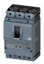
circuit breaker 3VA2 IEC frame 160 breaking capacity class C Icu=110kA @ 415V 3-pole, line protection ETU330, LIG, In=63A overload protection Ir=25A...63A short-circuit protection Ii=1.5...12 x In ground-fault protection Ig=0.25... 1 x In, tg=0.1/0.3s clamp connection
