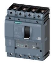
circuit breaker 3VA2 IEC frame 160 breaking capacity class C Icu=110kA @ 415V 4-pole, line protection ETU320, LI, In=63A overload protection Ir=25A...63A short-circuit protection Ii=1.5...12 x In N conductor protection adjustable (OFF, 100%) nut keeper kit
