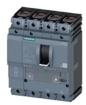
circuit breaker 3VA2 IEC frame 160 breaking capacity class C Icu=110kA @ 415V 4-pole, line protection ETU340, ELISA LI, In=63A overload protection Ir=25A...63A short-circuit protection Ii=15 x In N conductor protection adjustable (OFF, 100%) clamp connection
