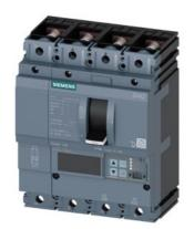
circuit breaker 3VA2 IEC frame 160 breaking capacity class H Icu=85kA @ 415V 4-pole, line protection ETU860, LSIG, In=63A overload protection Ir=25A...63A short-circuit protection Isd=0.6..10x In, Ii=1.5..12x In N conductor protection adjustable (OFF, up to 160%) gr.-fault prot., can be sw. off Ig=0.25...1 x In= tg=0.05-0.8s nut keeper kit
