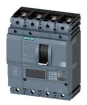
circuit breaker 3VA2 IEC frame 160 breaking capacity class H Icu=85kA @ 415V 4-pole, line protection ETU850, LSI, In=63A overload protection Ir=25A...63A short-circuit protection Isd=0.6..10x In, Ii=1.5..12x In N conductor protection adjustable (OFF, up to 160%) nut keeper kit
