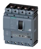
circuit breaker 3VA2 IEC frame 160 breaking capacity class H Icu=85kA @ 415V 4-pole, line protection ETU350, LSI, In=63A overload protection Ir=25A...63A short-circuit protection Isd=1.5...10 x Ir, Ii=12 x In N conductor protection adjustable (OFF, 100%) nut keeper kit
