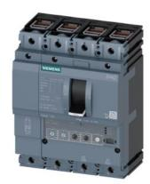
circuit breaker 3VA2 IEC frame 160 breaking capacity class H Icu=85kA @ 415V 4-pole, line protection ETU330, LIG, In=63A overload protection Ir=25A...63A short-circuit protection Ii=1.5...12 x In N conductor protection adjustable (OFF, 100%) ground-fault protection Ig=0.25...1 x In= tg=0.1/0.3s clamp connection
