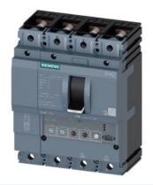
circuit breaker 3VA2 IEC frame 160 breaking capacity class H Icu=85kA @ 415V 4-pole, line protection ETU330, LIG, In=63A overload protection Ir=25A...63A short-circuit protection Ii=1.5...12 x In N conductor protection adjustable (OFF, 100%) ground-fault protection Ig=0.25...1 x In= tg=0.1/0.3s nut keeper kit
