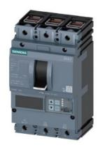
CIRCUIT BREAKER 3VA2 IEC FRAME 160 BREAKING CAPACITY CLASS C ICU=110KA @ 415 V 3-POLE, MOTOR PROTECTION ETU550M, LSI, In=40A OVERLOAD PROTECTION IR=16A ...40A SHORT CIRCUIT PROTECTION ISD=1,2... 15X IN,II=3...15X IN CABLE CONNECTION
