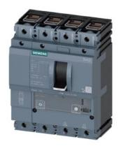
circuit breaker 3VA2 IEC frame 160 breaking capacity class C Icu=110kA @ 415V 4-pole, line protection ETU340, ELISA LI, In=40A overload protection Ir=16A...40A short-circuit protection Ii=15 x In N conductor protection adjustable (OFF, 100%) clamp connection
