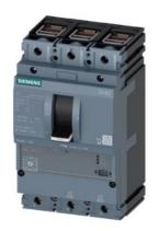
circuit breaker 3VA2 IEC frame 160 breaking capacity class C Icu=110kA @ 415V 3-pole, line protection ETU340, ELISA LI, In=40A overload protection Ir=16A...40A short-circuit protection Ii=15 x In clamp connection
