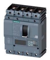
circuit breaker 3VA2 IEC frame 160 breaking capacity class H Icu=85kA @ 415V 4-pole, line protection ETU560, LSIG, ln=40A overload protection lr=16A...40A short-circuit protection Isd=0.6..10x In, li=1.5..12x In N conductor protection adjustable (OFF, up to 160%) gr.-fault prot., can be sw. off lg=0.4...1 x ln= tg=0.05-0.8s nut keeper kit
