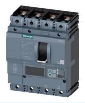
circuit breaker 3VA2 IEC frame 160 breaking capacity class H Icu=85kA @ 415V 4-pole, line protection ETU550, LSI, In=40A overload protection Ir=16A...40A short-circuit protection Isd=0.6..10x In, Ii=1.5..12x In N conductor protection adjustable (OFF, up to 160%) nut keeper kit
