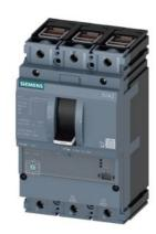
circuit breaker 3VA2 IEC frame 160 breaking capacity class H Icu=85kA @ 415V 3-pole, line protection ETU340, ELISA LI, In=40A overload protection Ir=16A...40A short-circuit protection Ii=15 x In clamp connection
