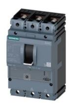
circuit breaker 3VA2 IEC frame 160 breaking capacity class C Icu=110kA @ 415V 3-pole, starter protection ETU310M, I, In=25A without overload protection short-circuit protection Ii=3...15 x In nut keeper kit
