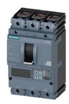
circuit breaker 3VA2 IEC frame 160 breaking capacity class C Icu=110kA @ 415V 3-pole, motor protection ETU860M, LSIG, In=25A overload protection Ir=10A...25A short-circuit protection Isd=1.2..15x In, Ii=3..15x In gr.-fault prot., can be sw. off Ig=0.6... 1 x In, tg=0.05-0.8s clamp connection
