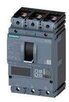
circuit breaker 3VA2 IEC frame 160 breaking capacity class C Icu=110kA @ 415V 3-pole, motor protection ETU860M, LSIG, In=25A overload protection Ir=10A...25A short-circuit protection Isd=1.2..15x In, Ii=3..15x In gr.-fault prot., can be sw. off Ig=0.6... 1 x In, tg=0.05-0.8s nut keeper kit
