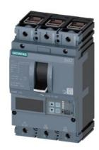
CIRCUIT BREAKER 3VA2 IEC FRAME 160 BREAKING CAPACITY CLASS C ICU=110KA @ 415 V 3-POLE, MOTOR PROTECTION ETU550M, LSI, In=25A OVERLOAD PROTECTION IR=10A ...25A SHORT CIRCUIT PROTECTION ISD=1,2... 15X IN,II=3...15X IN CABLE CONNECTION
