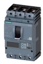
CIRCUIT BREAKER 3VA2 IEC FRAME 160 BREAKING CAPACITY CLASS C ICU=110KA @ 415 V 3-POLE, MOTOR PROTECTION ETU550M, LSI, In=25A OVERLOAD PROTECTION IR=10A ...25A SHORT CIRCUIT PROTECTION ISD=1,2... 15X IN,II=3...15X IN BUSBAR CONNECTION
