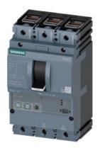
circuit breaker 3VA2 IEC frame 160 breaking capacity class C lcu=110kA @ 415V 3-pole, motor protection ETU350M, LSI, ln=25A overload protection Ir=10A...25A short-circuit protection Isd=3...15 x Ir, li=15 x In clamp connection
