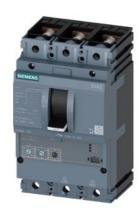
circuit breaker 3VA2 IEC frame 160 breaking capacity class C Icu=110kA @ 415V 3-pole, motor protection ETU350M, LSI, In=25A overload protection Ir=10A...25A short-circuit protection Isd=3...15 x Ir, Ii=15 x In nut keeper kit
