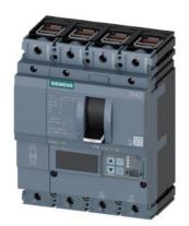
circuit breaker 3VA2 IEC frame 160 breaking capacity class C Icu=110kA @ 415V 4-pole, line protection ETU860, LSIG, In=25A overload protection Ir=10A...25A short-circuit protection Isd=0.6..10x In, Ii=1.5..12x In N conductor protection adjustable (OFF, up to 160%) gr.-fault prot., can be sw. off Ig=0.2...1 x In= tg=0.05-0.8s clamp connection
