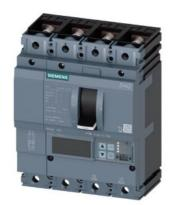
circuit breaker 3VA2 IEC frame 160 breaking capacity class C Icu=110kA @ 415V 4-pole, line protection ETU860, LSIG, In=25A overload protection Ir=10A...25A short-circuit protection Isd=0.6..10x In, Ii=1.5..12x In N conductor protection adjustable (OFF, up to 160%) gr.-fault prot., can be sw. off Ig=0.2...1 x In= tg=0.05-0.8s nut keeper kit
